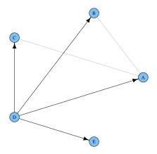
The default layout algorithm is igraph::layout.circle, other layout algorithms can be used by passing them as an optional argument called layout to plot. The igraph::layout.fruchterman.reingold algorithm also seems to produce nice results and may be better for large graphs.
