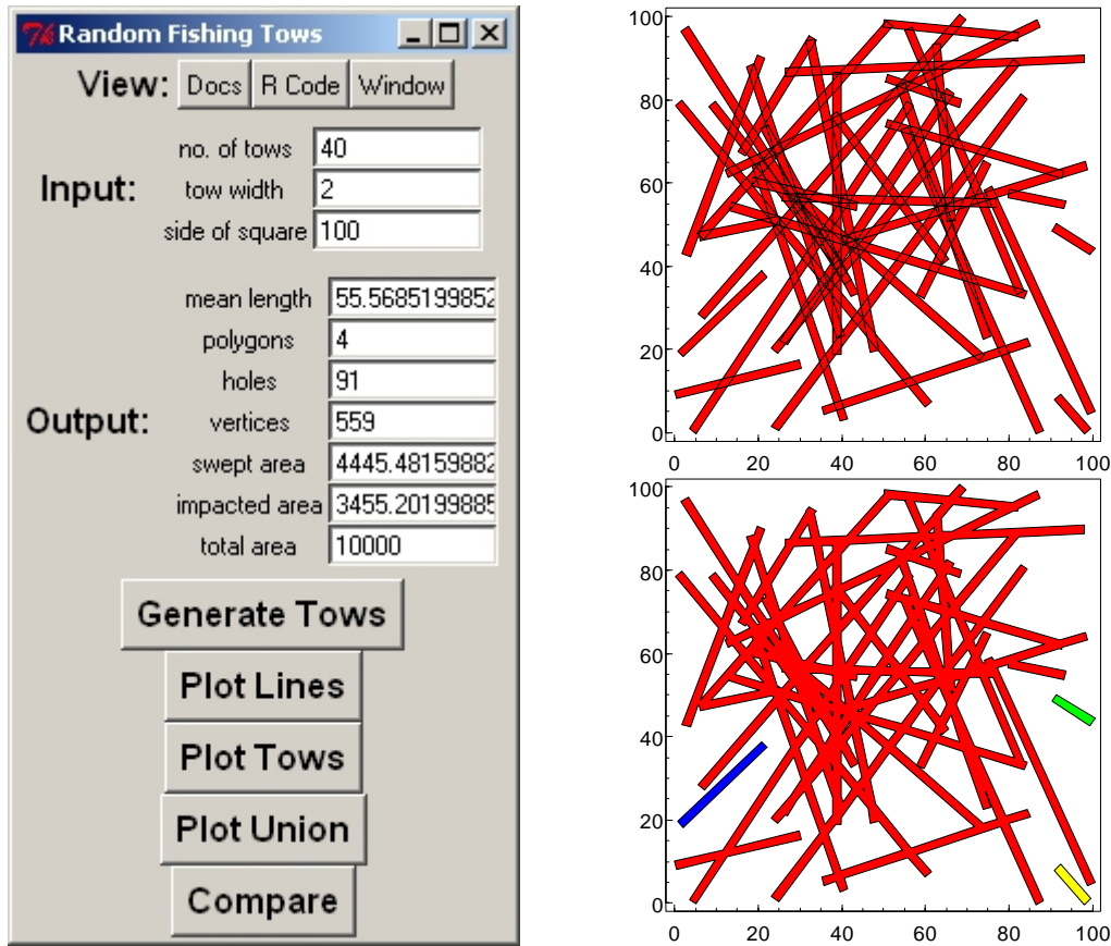
Figure 13. FishTows GUI (left) and simulated tow track (right). Tow track plots show 40 random tows in a square with side length 100. Each tow has width 2, and the rectangle encompasses 10,000 square units. Top: The individual rectangles, with 160 vertices, have areas that sum to 4,445 square units. Bottom: The union includes a complex polygon (red) and three isolated rectangles (blue, green, yellow) that cover only 3,455 square units. The complex polygon (red) has 547 vertices and 91 holes.
